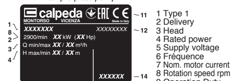
Example plate motor
