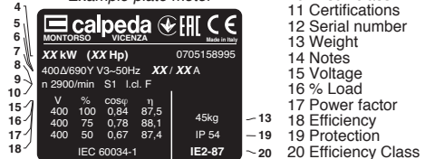
Example plate motor
