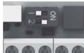
Fig. 3 Cutting the termination resistor in and out
