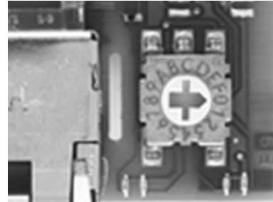
Fig. 16 Selecting the Industrial Ethernet protocol
