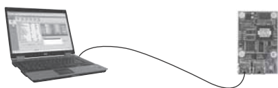
Fig. 17 CIM 500 connected to PC via Ethernet cable
