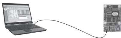
Fig. 13 CIM 500 connected to PC via ethernet cable
