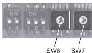
Fig. 8 Setting the BACnet MAC address
