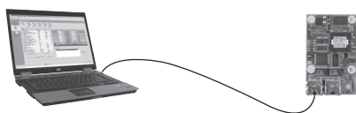
Fig. 17 CIM 500 connected to PC via Ethernet cable
