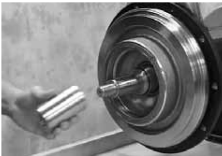
Fig. 13 Removing positioning tool
