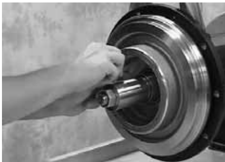
Fig. 12 Tightening shaft seal
