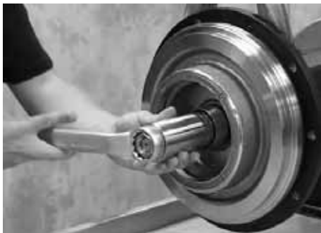
Fig. 11 Positioning tool for primary shaft seal
