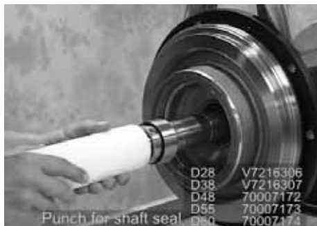
Fig. 7 Punching for shaft seal
