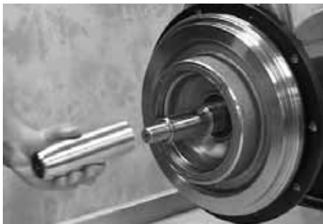
Fig. 3 Fitting protective sleeve
