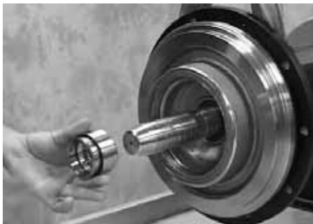
Fig. 6 Fitting shaft seal on shaft
